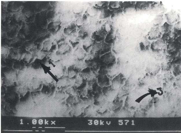
Figure 5. Enamel etched for sixty seconds with phosphoric acid. Arrow (1) indicates type I etch-pattern. Arrow (right) shows type III etch-pattern.
