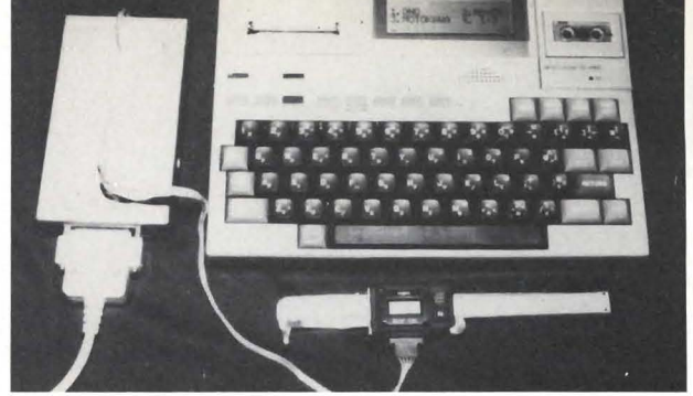
Figure 2. Handheld computer, measure interface and caliper.
