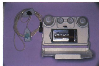
Figure 1. The 3M Dental Electronic Anesthesia System (8670) is shown. The large outside knobs are amplitude controls, and the small inside knobs control pulse rate and pulse width. Lead wires are connected to the unit on the left. Manufacturer's description of all controls should be studied carefully before use.
