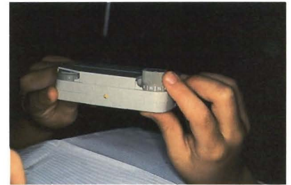
Figure 13. For most dental restorative procedures, the amplitude control knob reaches a setting of between 10 and 20. Some treatment, with some patients, can be performed with a setting as low as 10, but muscular fasciculation should be seen, as a sign of reaching minimum therapeutic dose level.
