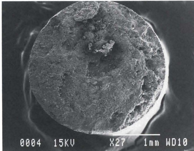
Figure 8. Specimen in Group 5 (no glaze, no polish, APF gel). This group reveals the effect of the APF gel on the micromorphology of the glass ionomer cement. Characteristics of an etched glass ionomer cement, with glass particles protruding from the surface, are evident in these illustrations.
