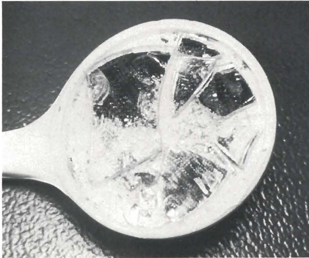
Figure 1. The fragmented mirrored surface of the "plastic" dental mirror after being bitten.
