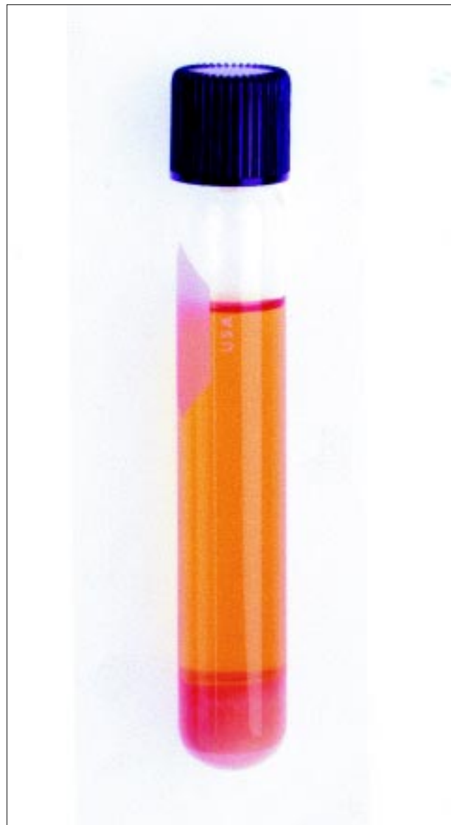
Fig 5. Sedimentation of NaF in test tube. (Reproduced with kind permission of Omnii Products®).
