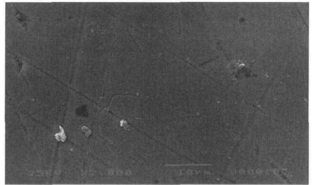
Fig 4. Scanning electron micrograph showing stainless steel crown surface in group 1 (adhesive failure) following debonding (2000x).
