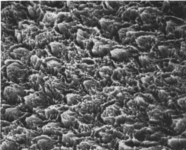
Figure 2. Scanning electron micrograph showing Type 2 etching pattern after applying phosphoric acid for 1 minute. (Magnification X 1750).
