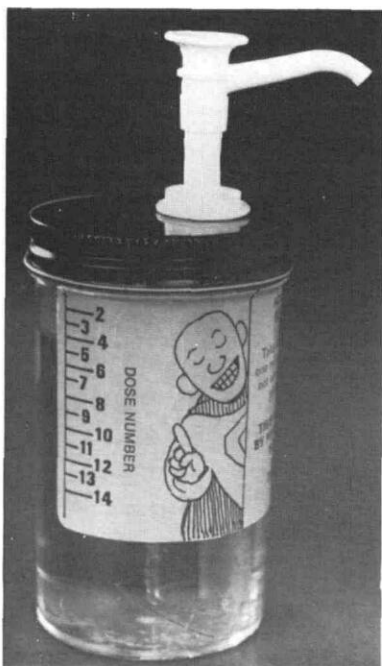
FIG 1. The principal dependent measure of compliance, number of doses of mouthrinse used, was measured from this dispensing bottle consisting of an outer bottle with an inner reservoir used to measure each dose. The pump releases only a single dose from the inner chamber every 8 - 14 hr. The number of doses used was measured from the label. The bottle could not be opened without breaking the DO NOT OPEN TAP AND TEARING THE LABEL.
