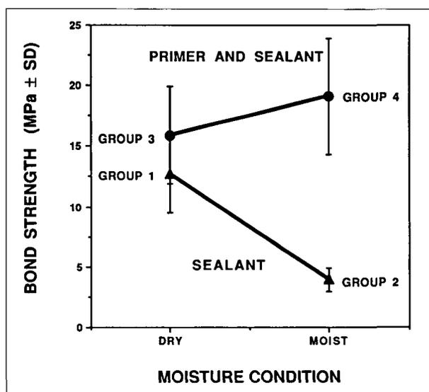
**Figure. Mean shear strength of sealant and sealant with primer under dry and moist conditions.**
