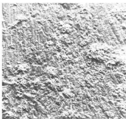
Figure 1. Scanning electromicrograph of the dentin surface after breaking the adhesive bond. The bond strength was 1,910 psi (13.2 MPa), and the fracture occurred partly at the interface (adhesive failure) and partly through the composite resin (cohesive failure) leaving remnants of the composite material adhering to the dentin surface. Original magnification 47x.
